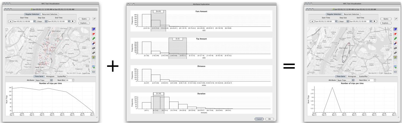
Fig. 6. Attribute constraints are specified (in the middle) to refine the query on the left. They are shown as dark gray strips on the histogram. The result of the refined query is shown on the right and consists of a single trip.
