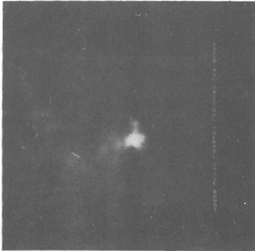
Fig. 10. Test image 1: 8-12- \mu m thermal image of size 200 \times 200 taken at Grafenwoehr, Germany. This image contains one object (white) at the center.
