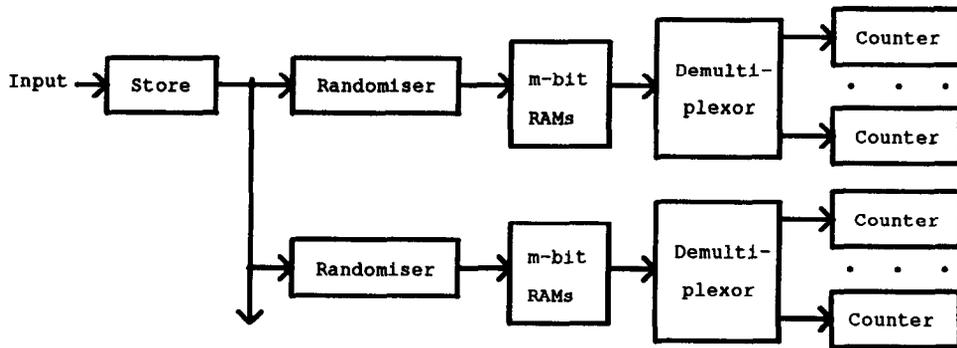
Fig. 9. Block diagram of 'coded memory' system.
