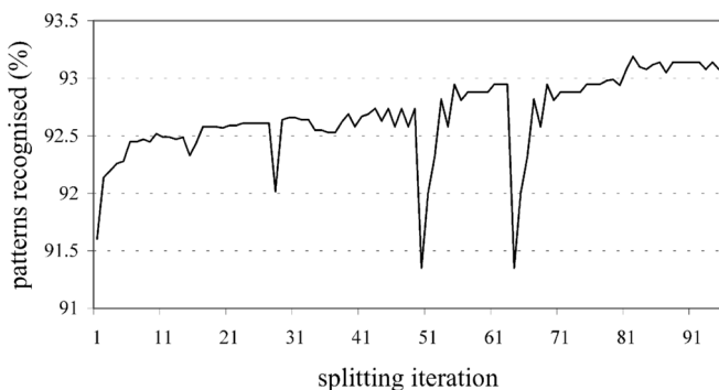
Fig. 6. The recognition rate of the system as it evolves from a 10-node system into a 15-node system. New nodes are introduced at iterations 1 (to separate class “1” from “2”), 15 (“1A” from “7”), 28 (“2” from “3”), 50 (“6” from “0”), and 64 (“3” from “5”).
