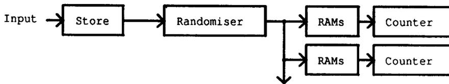
Fig. 4. Block diagram of multiple discriminator system.
